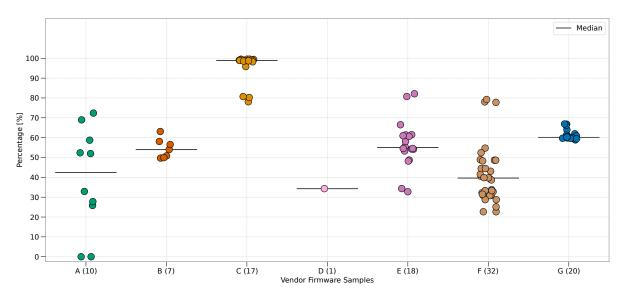
Figure 3.8: Percentage of Executables with PIE Enabled per Firmware Image
