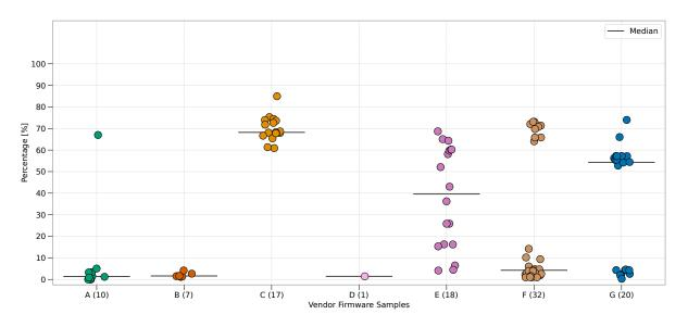
Figure 3.9: Percentage of Executables with RELRO Enabled per Firmware Image
