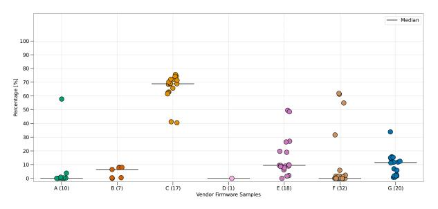
Figure 3.10: Percentage of Executables with Canary Enabled per Firmware Image
